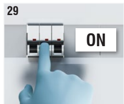
Fig. 29. Act on the safety magnetothermic switch positioned on the circuit upstream of the device to restore the electrical power supply.
