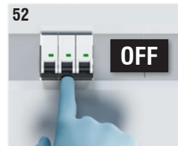
Fig. 52: Disconnect the power supply by acting on the safety thermomagnetic circuit upstream of the device. Make sure that the power supply cannot be accidentally restored.
