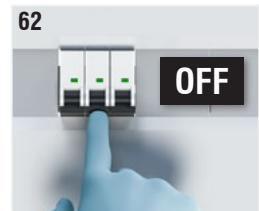
Fig. 62: Disconnect the power supply by acting on the safety thermomagnetic circuit upstream of the device. Make sure that the power supply cannot be accidentally restored.
