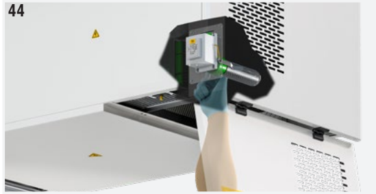
Fig. 44: Gently unscrew the ionising pipe, gripping it at the base (green part).
