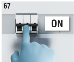
Fig. 67. Act on the safety magnetothermic switch positioned on the circuit upstream of the device to restore the electrical power supply.
