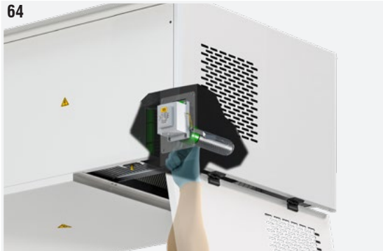
Fig. 64: Gently unscrew the ionising pipe, gripping it at the base (green part).
