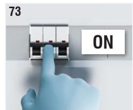
Fig. 73: Act on the safety magnetothermic switch positioned on the circuit upstream of the device to restore the electrical power supply.
