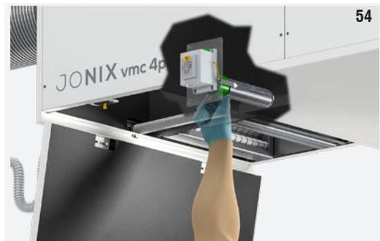
Fig. 54: Gently unscrew the ionising pipe, gripping it at the base (green part).
