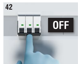
Fig. 42: Disconnect the power supply by acting on the safety thermomagnetic circuit upstream of the device. Make sure that the power supply cannot be accidentally restored.
