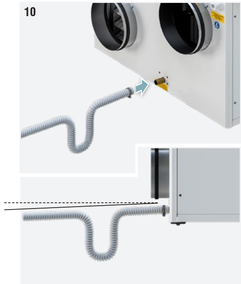
Fig. 10. Install the condensate drain with a flexible rubber hose and a minimum internal diameter of 16 mm. Create a siphon on the exhaust pipe with a head at least equal to the suction head of the fan. The condensate drain must be insulated if it passes through unheated spaces to prevent freezing.
