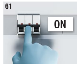
Fig. 61. Act on the safety magnetothermic switch positioned on the circuit upstream of the device to restore the electrical power supply.
